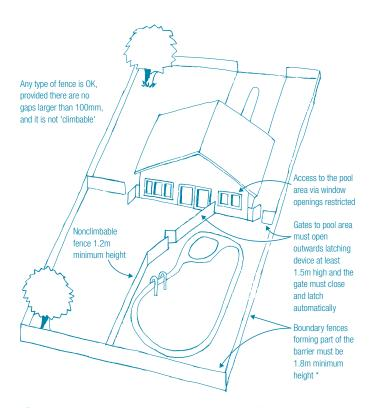
Boundary fences forming part of the barrier must be 1.8m high, with a 900mm non-climbable zone at the top on the pool side of the fence.
